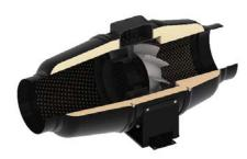
The conic impeller with special blade profiling increase air flow speed and provide higher pressure and air capacity as compared to standard axial fans. The diffuser, the specially profiled impeller and the directing vanes at outlet from the fan casing distribute air flow in such a way as to attain the best combination of high performance and high pressure at low noise level. The fan casing is equipped with an airtight terminal box for connection to power mains.
